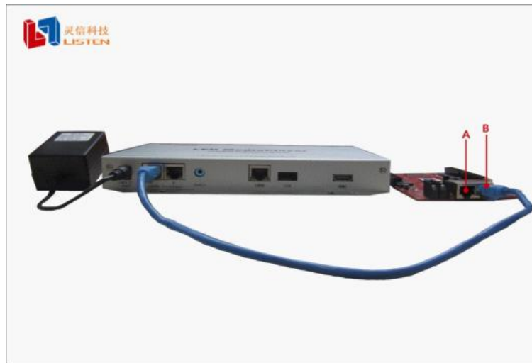
Cascade connection diagram for the receiving cards
